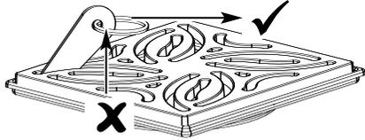
Apply sealant to underside of outer rim and install into centre hole of Tuff Form Former.
